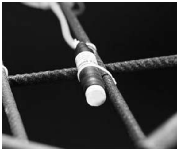
16.6 MnO 2 -reference electrode for measuring the potential of the steel attached to the reinforcement (ERE 20, Force Technology).
