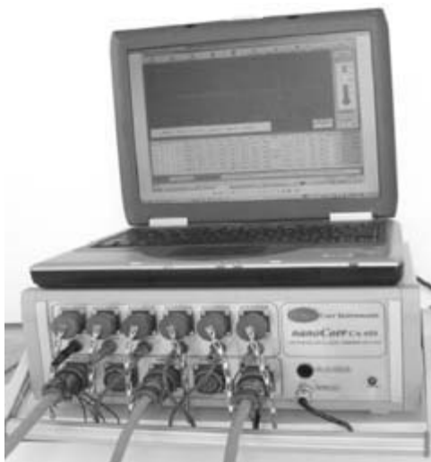
26.1 Typical coupled multielectrode array sensor analyzers for corrosion monitoring of cathodically protected systems, courtesy of Corr Instruments LLC.
