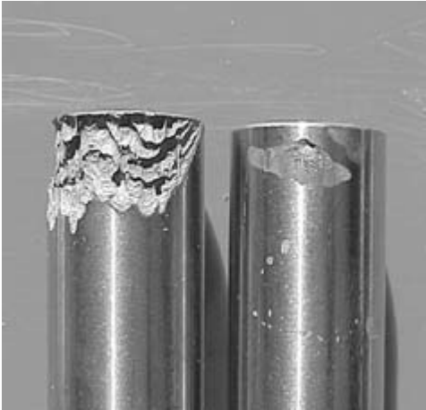
15.9 Crevice corrosion propagation on AISI 316 pipes after 3 months of exposure to untreated (left side) and automatically chlorinated seawater (right side) Mollica and Scotto (1996).
