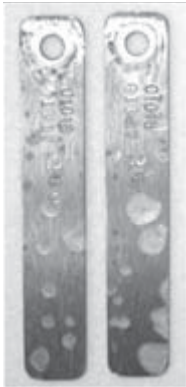
Coupon tests showed 100 to 200 mil/y (2.5 to 5 mm/y) pitting rate
