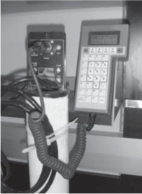
17.8 Portable ER instrument connected to SCP test station.
