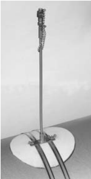
13.2 A commercial hydrogen flux probe (Hydrosteel® 6000, AT-S, Ion Science Ltd, UK). An analyser is attached to the central capillary and air drawn through it as described in the text. The probe, about 6 in. (15cm) diameter, is flexible and can tolerate steel temperatures to at least 500°C. Photograph courtesy Ion Science Ltd, UK.
