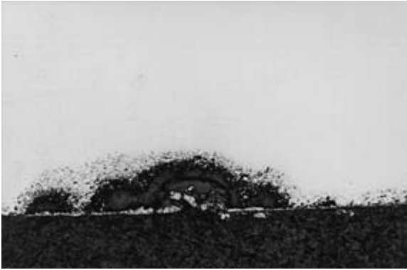
23.12 Bowl-shape depressions (i.e., under-deposit corrosion sites) beneath the red deposit layers on the condenser tube internal surface. Magnification: 50 \times .
