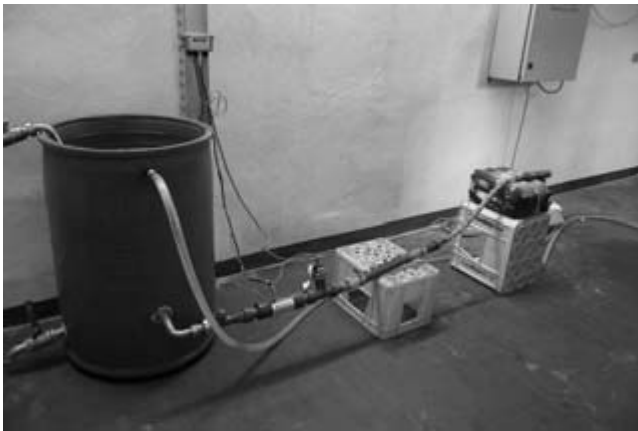
15.11 On-line monitoring of biofilm absence in mineral water plant by the BIOX system (Eurotherm77, 2005 with permission).
