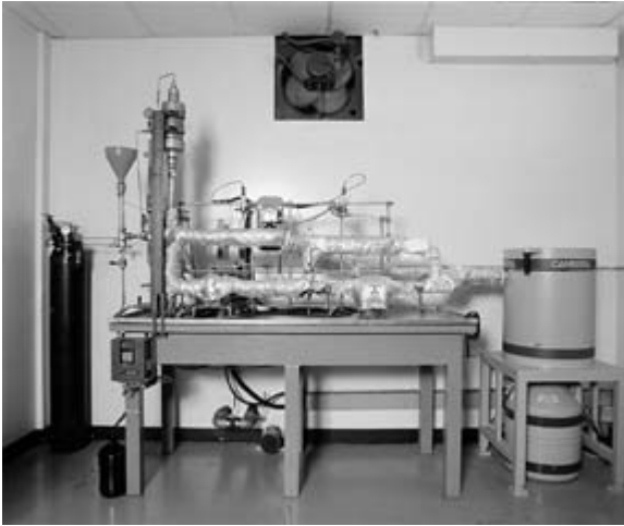
10.5 Real-time corrosivity measurement flow loop, courtesy Southwest Research Institute.
